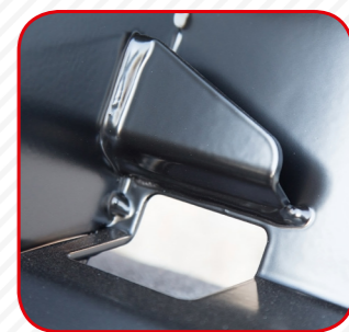
Reinforced hi-lift jacking points
